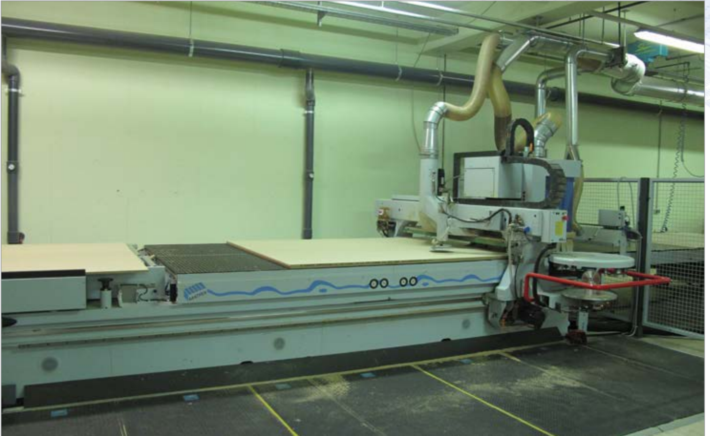
Fig. 1: One of the two CNC processing centers with NBM clamping tables.
