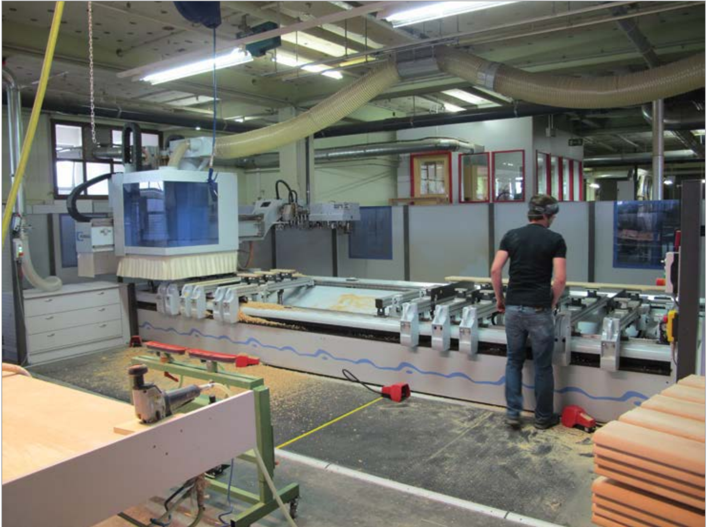
Fig. 4: CNC processing centre for solid wood processing at ADA.
