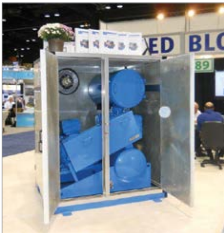
The United Blower “Quiet-Pulse” three-lobe, heavy-duty PD blower on display at WEFTEC.
