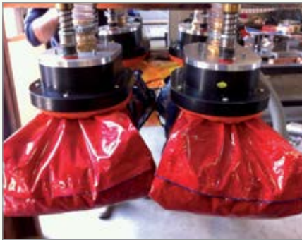
Piab's Kenos range of suction pad grippers are perfect for packaging and palletizing.
