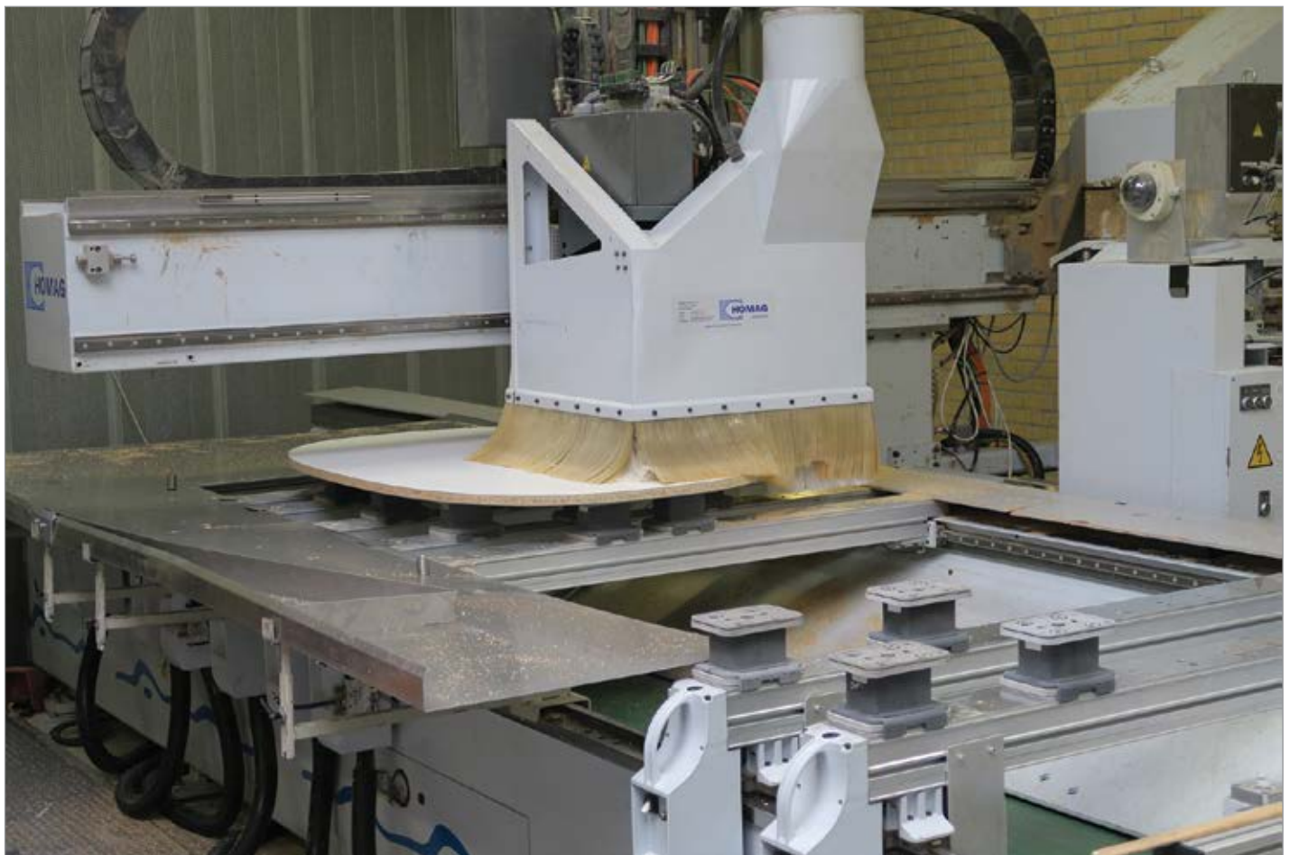
Figure 2. Solid wood and molded wood components are processed on several CNC machines.
