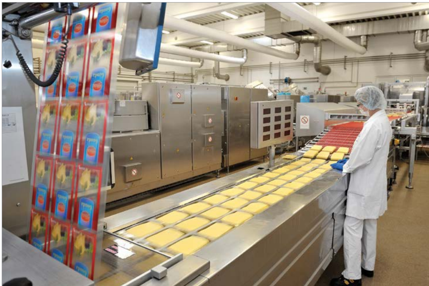
Figure 1: Cheese production at DMK in Georgsmarienhütte: packaging of sliced cheese with a thermoforming packaging machine.
