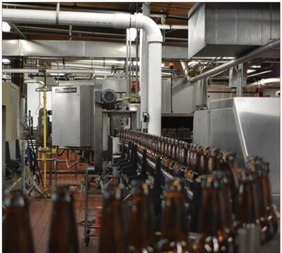
Widmer Brothers' bottling line produces up to 550 bottles per minute.
