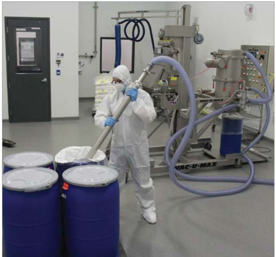
The process at A&C involves the use of a vacuum receiver mounted on mobile cart with attached pick-up adapter to convey powders.
