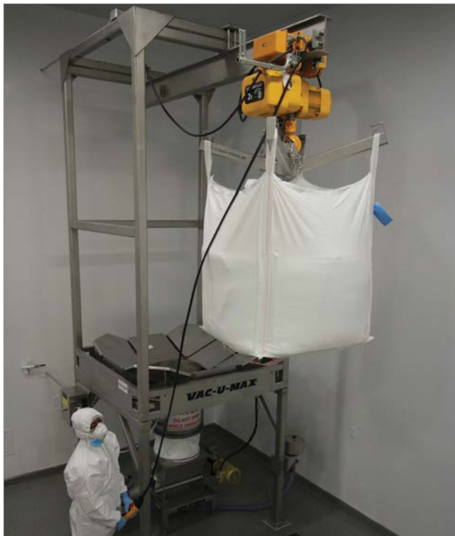
The Activator system features lubrication-free pneumatic lifters that consume 50% less compressed air than air-cylinders.
