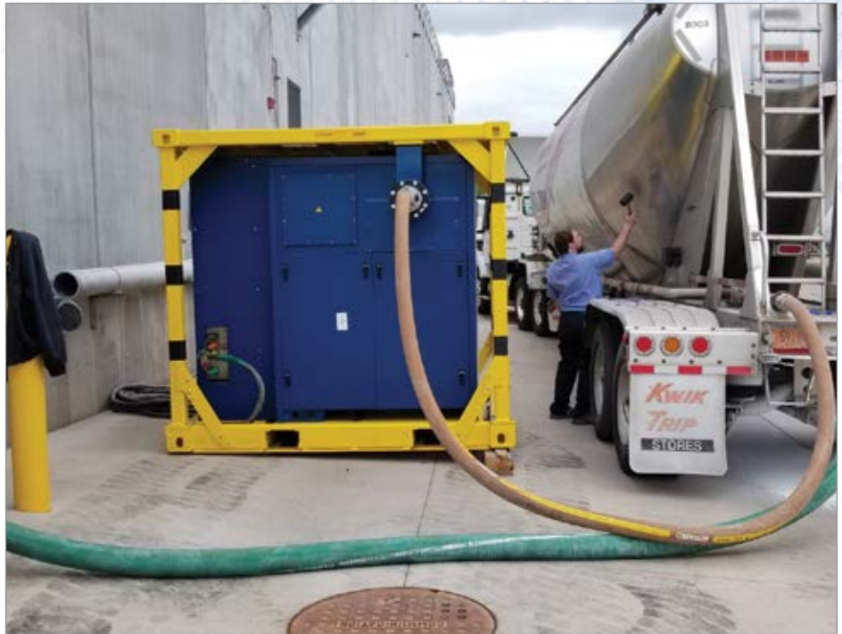
A bakery reduced truck offload time by replacing the wrong blower with a single-stage, oil-free rotary screw rental air compressor.
