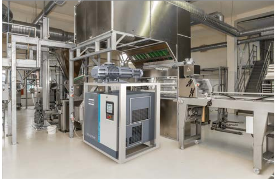
An Atlas Copco GHS VSD+ with a ZRS Mechanical Booster Pump. These booster pumps are suitable for use with high differential pressures which allow the booster pump to be started at the same time as the backing pump, reducing total pump down times.
