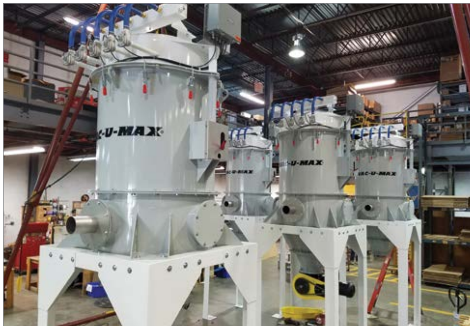
Filter receivers (filter separators) ready to be shipped to the tea manufacturer.
