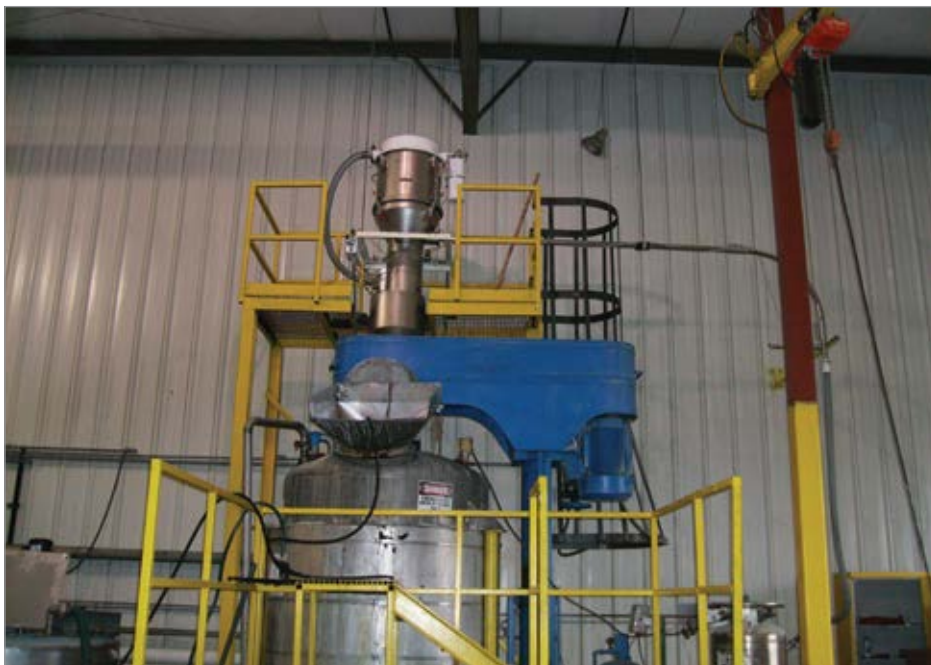
Pneumatic systems, like this one by VAC-U-MAX, convey material from closed hoppers through closed lines and requires little to no intervention.
