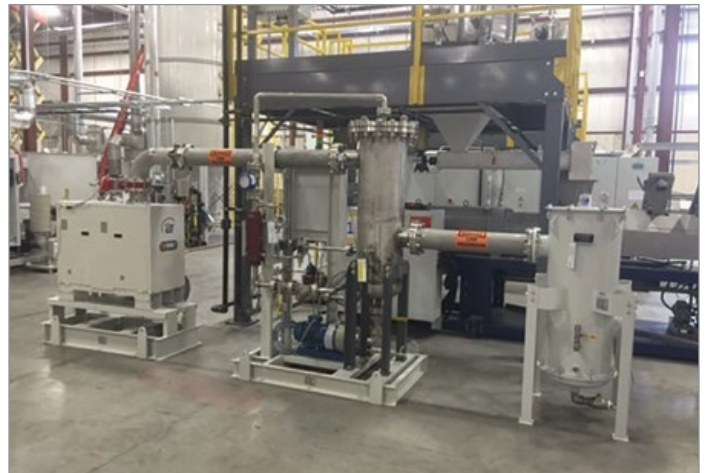
High performance vacuum system with dry screw/booster, scrubber system, and knockout pot.
